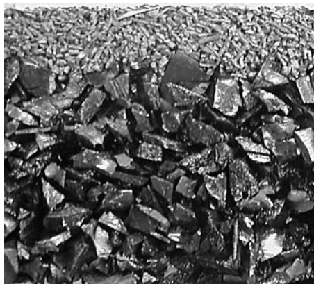
Figure 1 Cross section of rubber based impact absorbing bilaminate material 4 with 6.0 cm base and 1.5 cm top layer.
